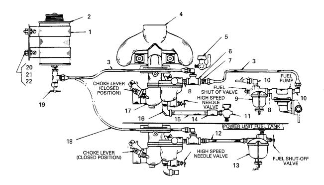
Engines which are to operate on No. 1 fuel oil of 38-42° Baume and an Octane rating of 35 or better, or kerosene, must be fitted with low compression cylinder heads and special fittings in carburetor. Do not use this fuel in a standard engine.
