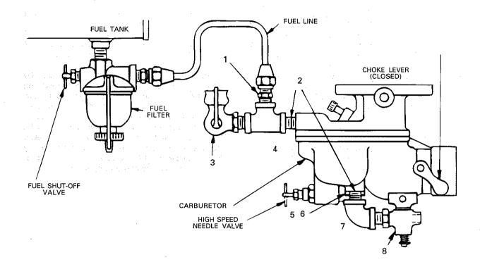
Engines which are to operate on No. 1 fuel oil of 38-42° Baume and an Octane rating of 35 or better, or kerosene, must be fitted with low compression heads and special fittings in carburetor. Do not use this fuel in a standard engine.
