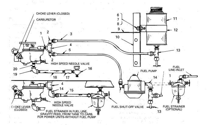
Engines which are to operate on No. 1 fuel oil of 38-42° Baume and an Octane rating of 35 or better, or kerosene, must be fitted with low compression cylinder heads and special fittings in carburetor. Do not use this fuel in a standard engine.
